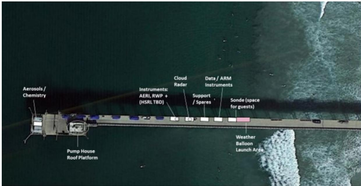
*Figure 2. ARM container layout on Scripps Pier.*
