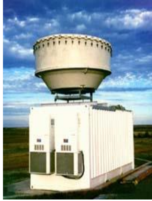
Fig. 2 - Millimeter Wave Cloud Radar (Credit - ARM)
