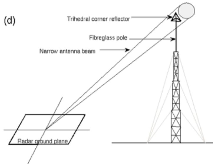
**Figure 9.** Calibration target.
