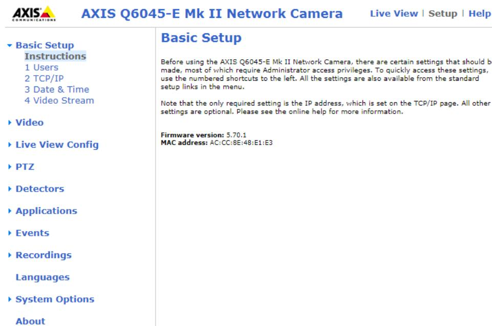
**Figure 9.** AXIS camera can be configured underneath the ‘Setup’ menu on the AXIS GUI. The toolbar on the left side of the page shows the variety of features that can be configured.
