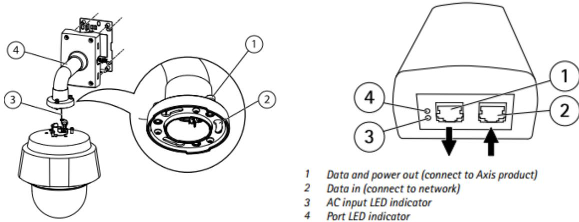
**Figure 6.** Camera and midspan installation diagrams from AXIS Q6045-E Mk II Installation Guide.
