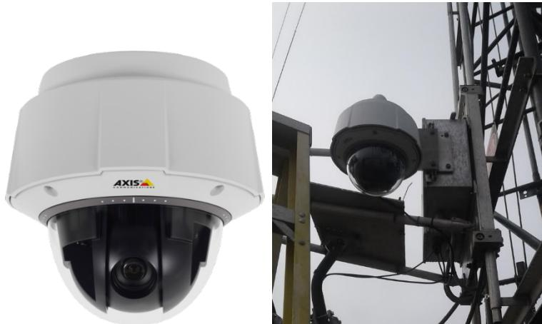
**Figure 2.** The AXIS Q6045-E Mk II PTZ Dome Network Camera currently installed on the topmost boom of the NSA-C1 40m tower.
