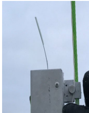
Figure 11. Anasphere SLWC sonde on TBS tether.
