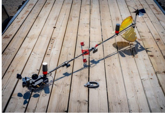
Figure 12. TBS wind sensor boom with vertical wind and cup anemometers and wind direction antennas.
