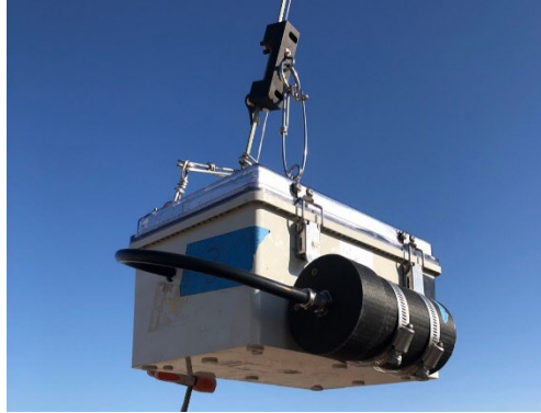
Figure 5. TSI CPC 3007 in flight with diffusion dryer.
