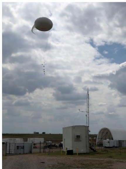
Figure 1. TBS using 122 m 3 aerostat in flight at SGP in September 2023.
