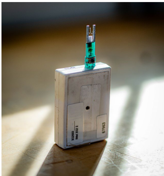
Figure 9. iMet XQ2 sensor used on ARM TBS.
