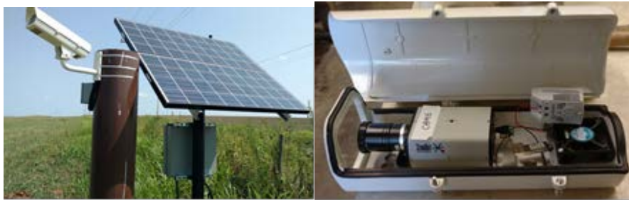
Figure 1. (Left) STEREOCAM in use at the ARM SGP site. (Right) STEREOCAM in carrying case.
