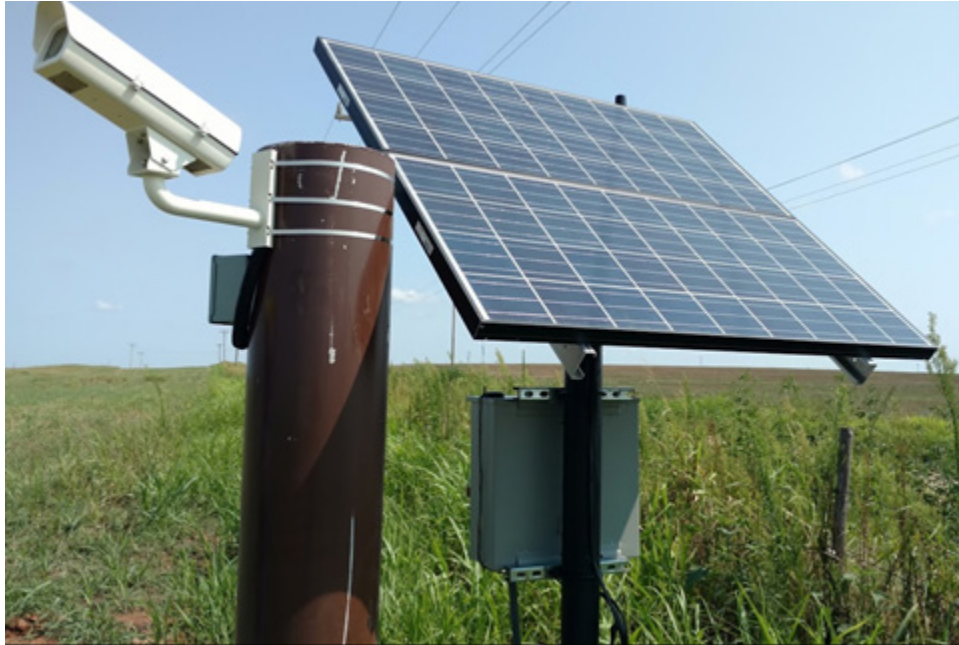
Figure 2. A camera setup onsite. Two solar panels mounted with a top-of-pole rack, an electrical enclosure beneath the solar panels, and the camera enclosure tilted approximately 18^\circ from the ground.
