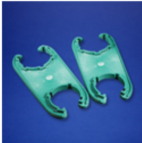
Figure 11. 47-mm filter holder wrenches.
