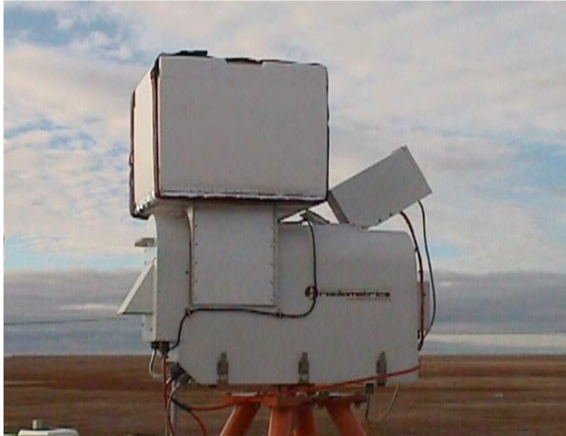
**Figure 2.** The microwave Radiometer Profiler (MWRP) at Barrow, Alaska with the LN2-filled Styrofoam target in place during calibration of the V-band channels in September 2000.
