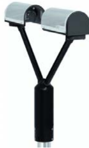
Figure 2. Parsivel2 device. The transmitter is located in one housing and the detector in the other.
