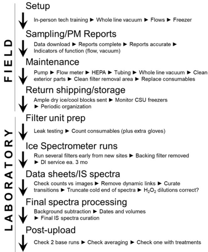
**Figure 5.** Flow diagram of QA/QC protocols designed for INPs. Quality assurance ensures quality requirements are fulfilled for both ARM management and end users. Quality control maintains quality requirements via inspection and testing to ensure performance characteristics conform to pre-specified requirements.
