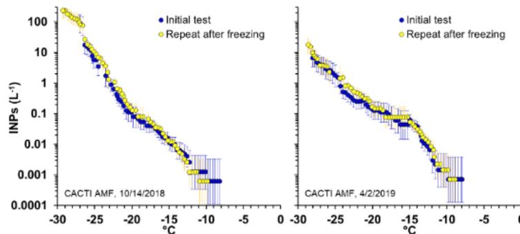
**Figure 6.** Repeatability of INP tests using suspensions that were tested immediately after re-suspension of particles from filters, then re-tested after frozen storage of the suspension (tubes were briefly pulse-vortexed after thawing). Vertical bars are 95% confidence intervals.
