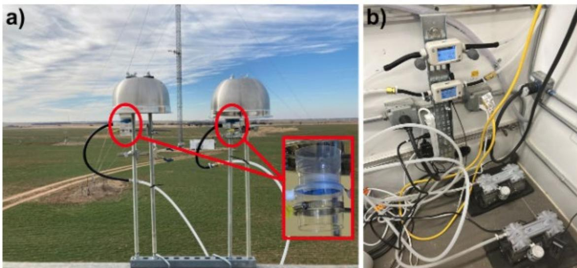
**Figure 1.** Filter unit sampling apparatuses, including a) single-use filter units under precipitation shields that are connected via tubing to b) the mass flow meters and vacuum pumps. The inset in a) shows a magnified photo of a filter unit. Photos in a) and b) are from ARM’s Southern Great Plains (SGP) observatory in Oklahoma and the Surface Atmosphere Integrated Field Laboratory (SAIL) site in Colorado, respectively.
