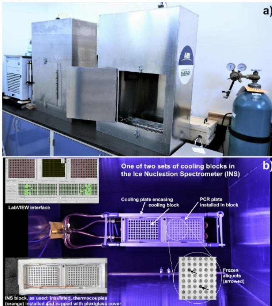
**Figure 2.** The INS, including: a) a photo of the exterior showing both cooling systems, one with the door open exposing the cooling blocks for scale and b) interior view of one system. PCR trays are loaded into the cooling blocks, the headspace purged with cooled and high-efficiency particulate air (HEPA)-filtered air, blocks cooled at  $0.33\text{ }^{\circ}\text{C min}^{-1}$ , and freezing events logged automatically through a LabVIEW interface with a camera.
