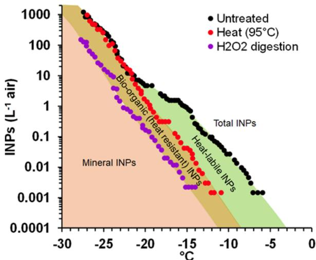
**Figure 9.** Cumulative INP spectra from a filter collected during the ARM CACTI campaign. Spectra include total INPs in addition to unique treatments that differential heat-labile (proteinaceous), heat-resistant (bio-organic), and mineral INP concentrations.
