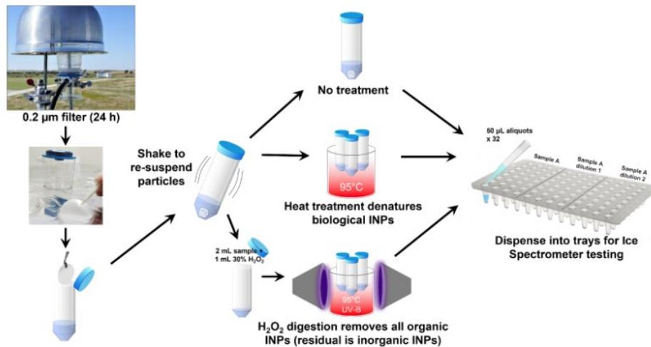
**Figure 3.** Schematic of workflow used to prepare samples for INP measurement in the INS.
