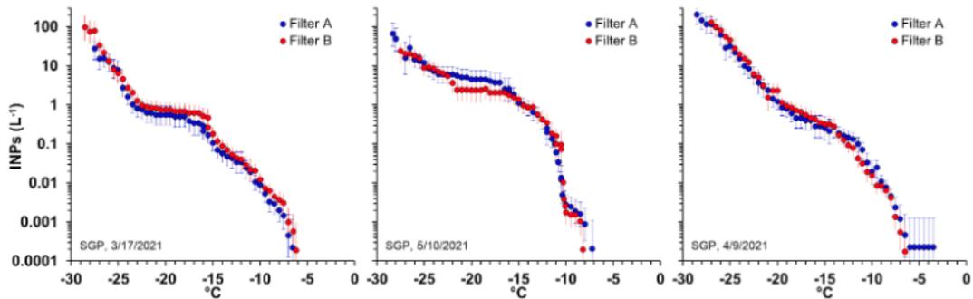
**Figure 7.** Comparability of INP spectra obtained from replicate filters taken at SGP. Vertical bars are 95% confidence intervals.
