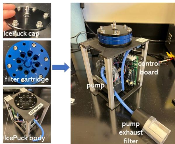
**Figure 4.** Images of some of the components of IcePuck and of the IcePuck assembled.
