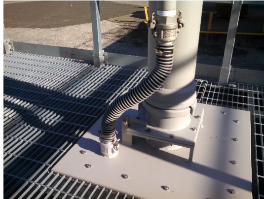
Figure 4. The base of the aerosol inlet, where it mates to the roof of the mobile laboratory.
