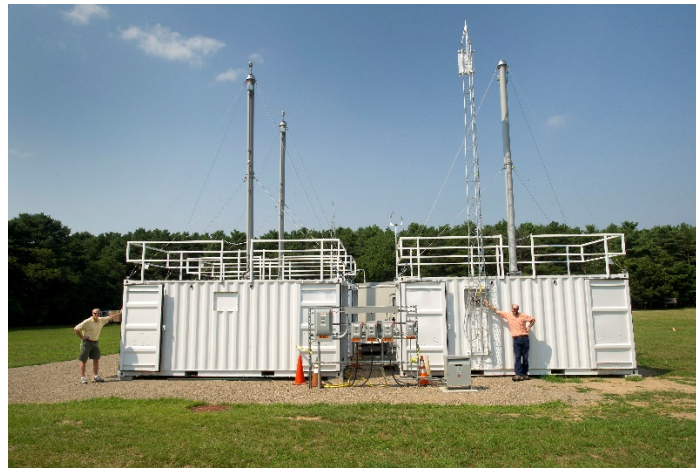
Figure 2. Multiple Aerosol Observing Systems side by side during an intercomparison at BNL, summer of 2010: (left) MAOS-A; (right) MAOS-C; (left rear) AOS06.
