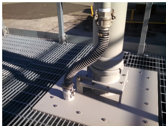
Figure 4. The base of the aerosol inlet, where it mates to the roof of the mobile laboratory.
