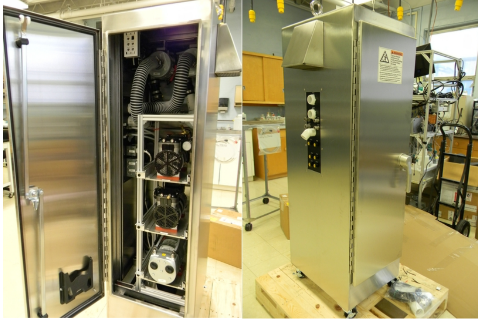
Figure 5. The AMF2 AOS blower enclosure interior and exterior.
