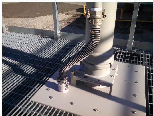
Figure 3. The base of the aerosol inlet, where it mates to the roof of the mobile laboratory.
