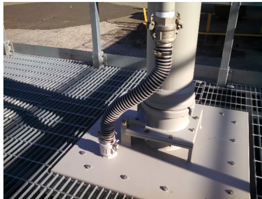
Figure 3. The base of the aerosol inlet, where it mates to the roof of the mobile laboratory.
