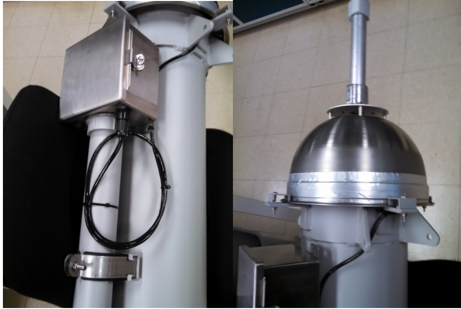
Figure 2. The junction box and the rain hat at the top of the aerosol inlet.
