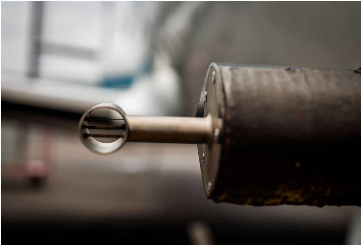
Figure 1. The sensor of the multi-element water content system.
