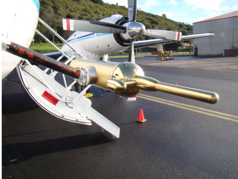
Figure 1. AIMMS probe installed on the U.S. Department of Energy’s Atmospheric Radiation Measurement (ARM) former Gulfstream-159 (G-1) aircraft.
