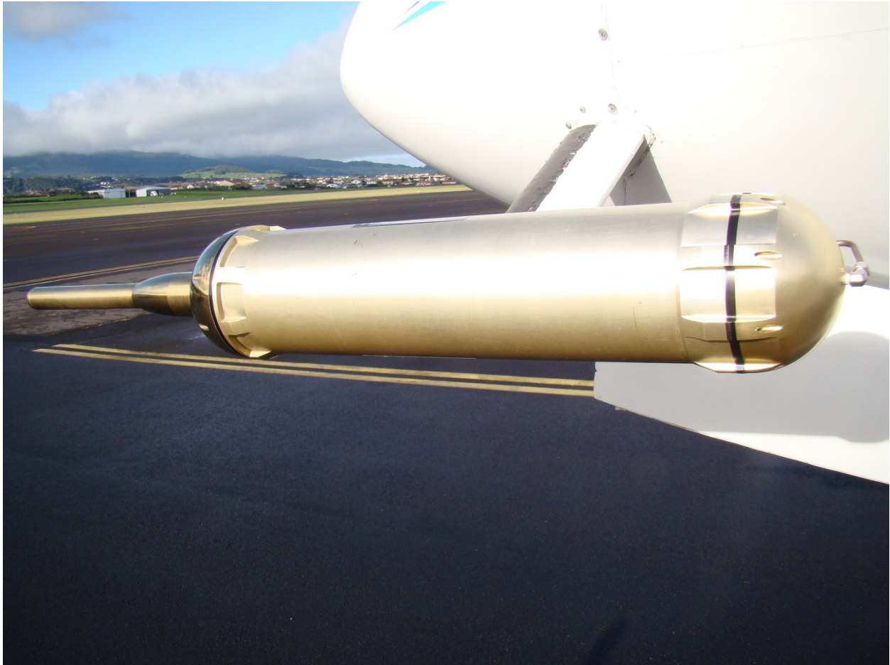
Figure 2. AIMMS probe canister housing mounted on the ARM G-1 aircraft.
