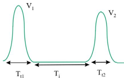
**Figure 4.** Imaging demonstrating particle inter-arrival time and the signal response from the detectors as seen on an oscilloscope taken from the DMT manual, Rev. F.
