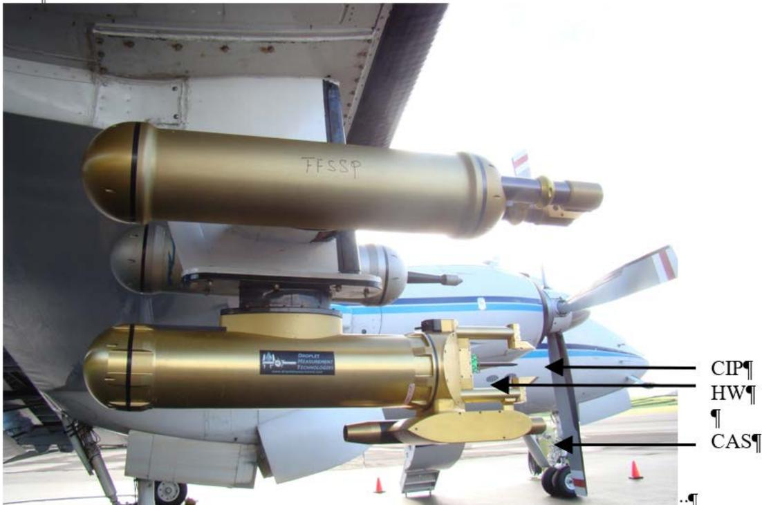
**Figure 1.** The U.S. Department of Energy Atmospheric Radiation Measurement (ARM) user facility Aerial Facility (AAF) pylon configuration with the CAPS instrument for the Aerosol and Cloud Experiments in the Eastern North Atlantic (ACE-ENA) campaign, 2018.
