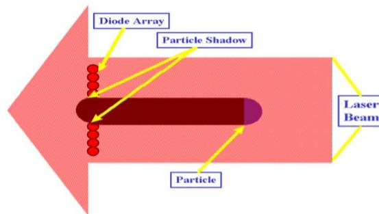
**Figure 6.** Representation of CIP theory of operation from the DMT manual, Rev. F.
