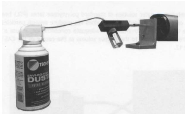
**Figure 8.** Glass bead calibration system for calibrations and tests. Image taken from 2010 vendor instrument manual uses a duster can instead of compressed air.
