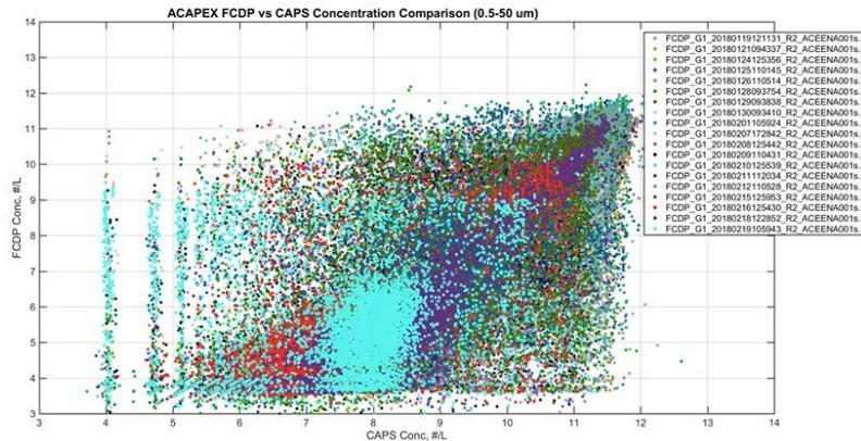
**Figure 2.** One-to-one comparison of total concentration of CAPS to fast cloud droplet probe (FCDP) during the ARM Cloud Aerosol Precipitation Experiment (ACAPEX). Data found and downloaded from ARM’s Data Center via “Data Discovery”.
