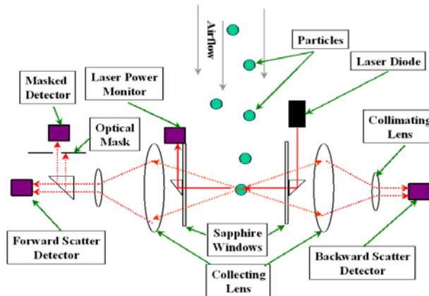
**Figure 5.** Schematic of forward and backscattering optical paths in the CAS from the DMT manual, Rev. F.
