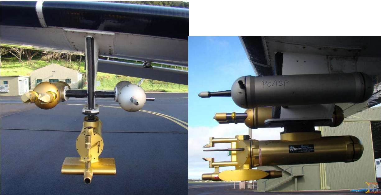
Figure 1. The PCASP is in the gray canister positioned on the starboard side of the aircraft under the wing.
