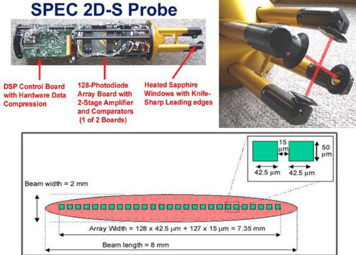
**Figure 5.** Photograph of 2D-S showing the probe (top left), the sample volume and laser beams (top right), and the setup of the beam illuminating the photodiode array (bottom). From the probe manual. (2)
