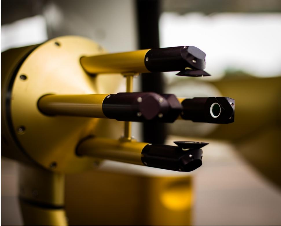
**Figure 1.** The two-dimensional stereo (2D-S) probe.
