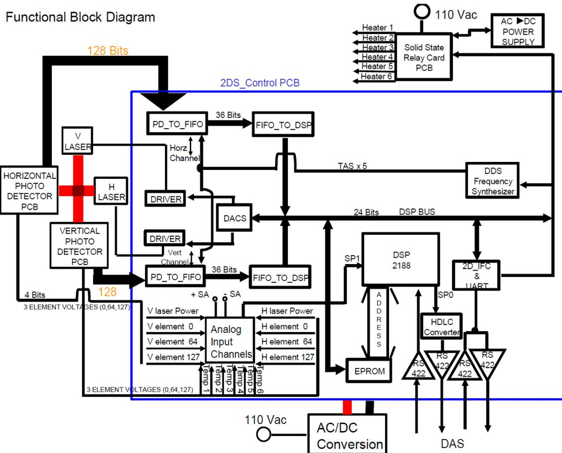
Figure 6. System block diagram provided by the vendor. Taken from the probe manual (2).
