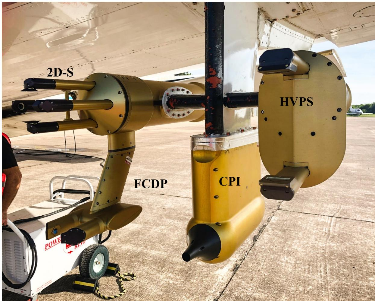
**Figure 7.** Mounting of several ARM cloud probes during CACTI. The 2D-S is located at the top left.
