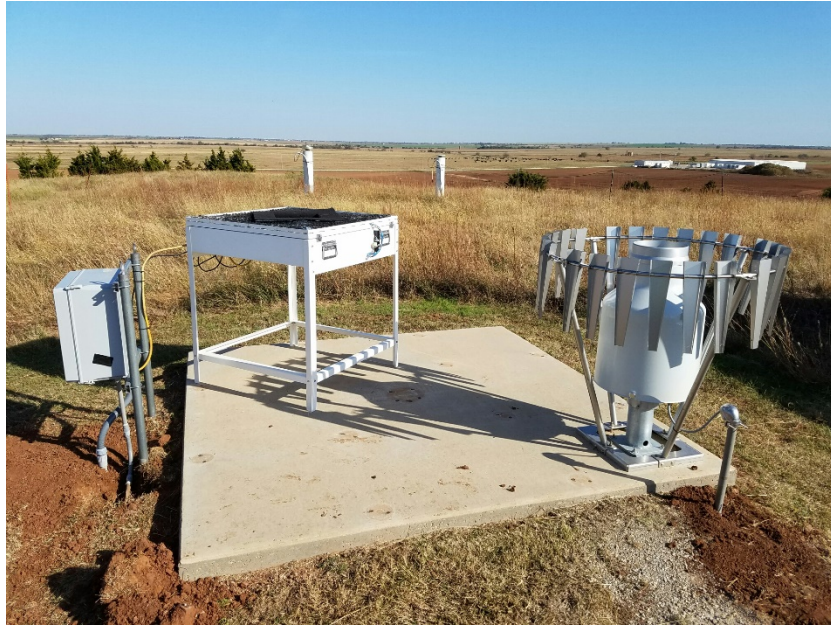
Figure 1. Two-dimensional video disdrometer on left; Pluvio2 weighing bucket rain gauge on right.
