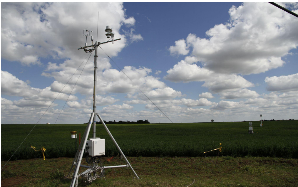
Figure 2. Photograph of 4 m tripod and soil and radiation satellites. Taken May 2018 by Sebastien Biraud .
