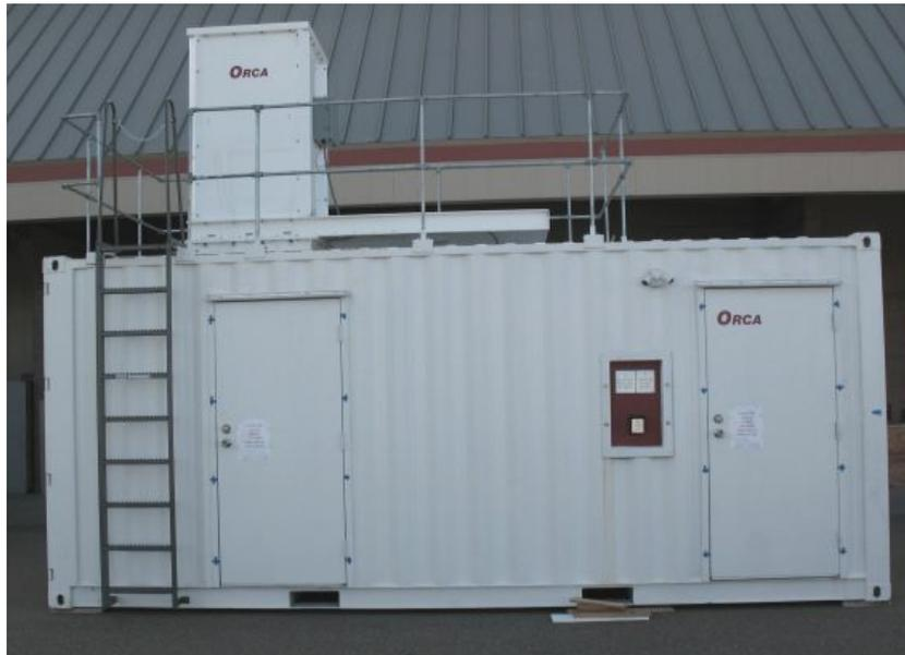
**Figure 1.** The ARM Raman lidar container. The laser beam exits through the light baffle on the top of the container.
