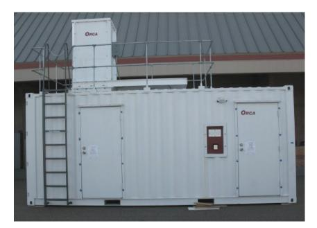
Figure 1. The ARM Raman lidar container. The laser beam exits through the light baffle on the top of the container.
