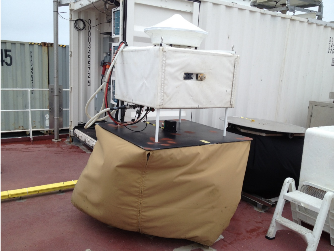
Figure 5. MWACR installed on RPH on board Horizon Spirit . Watson tilt sensor can be seen below MWACR, in center of table.
