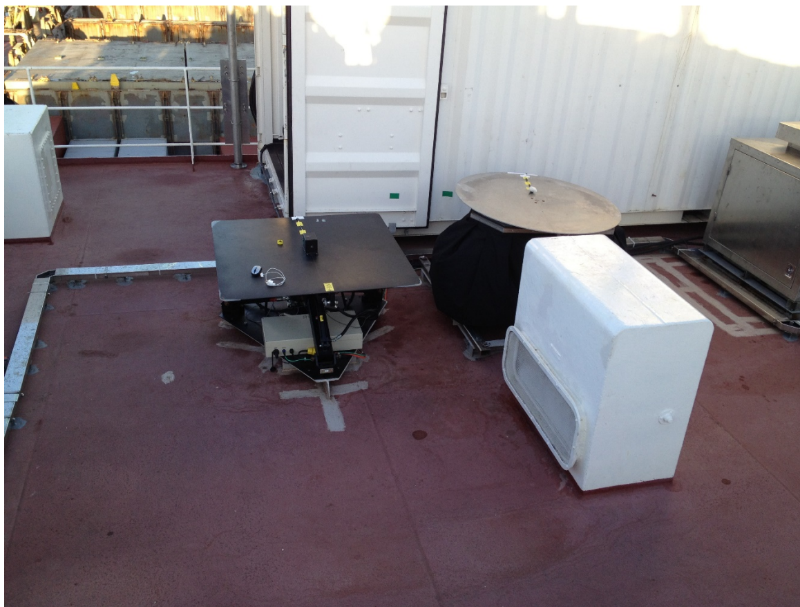
Figure 4. The RPH (left) and RPY (right) platforms during initial deployment. During this voyage, work with RPH was using SeaNav ship disposition data, which later was not available.
