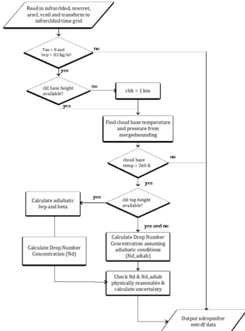
**Figure 1.** A flowchart of the NDROP VAP algorithm.
