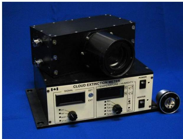
**Figure 2.** Cloud Extinction Probe: optical unit (top), control box (bottom), and retroreflector (right).
