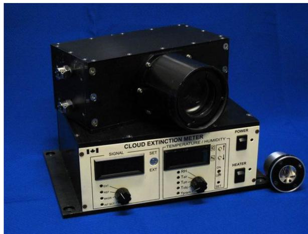
**Figure 2.** Cloud Extinction Probe: optical unit (top), control box (bottom), and retroreflector (right).
