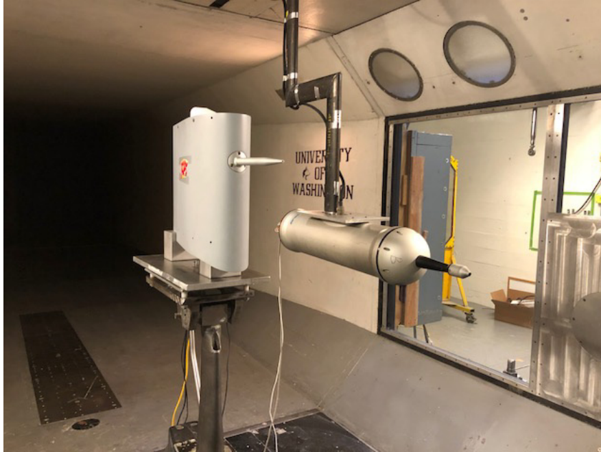
Figure 10. The pylon with POPS and inlet mounted on the main turntable inside the Kristen Wind Tunnel. The PCASP is mounted on a separate fixed arm.
