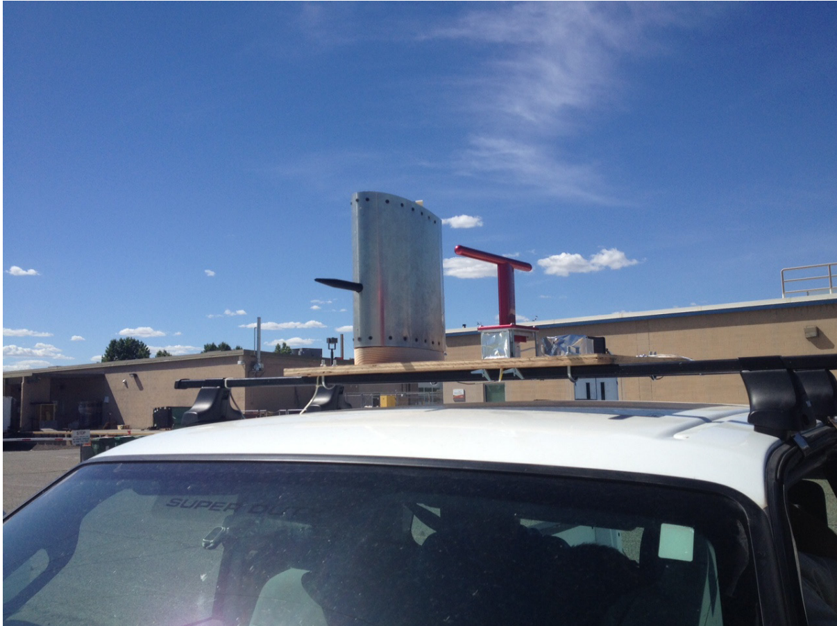
Figure 7. The POPS inlet prototype mounted in the mockup pylon on the cabin roof rack of a pickup truck. AIMMS-30 was mounted side by side with the inlets about 40 cm apart. NOTE: both pylon and AIMMS-30 were mounted upside down; normally, they hang down below a UAS wing.
