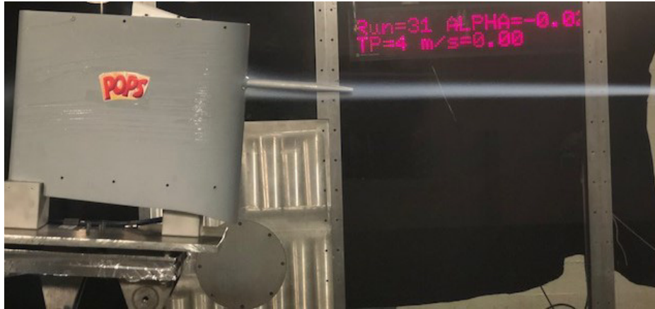
Figure 16. Example of smoke test ( AoA=-5^\circ , AoS=0^\circ , V_{air}=40 m/s) – note the inlet tip in the "straight and horizontal" part of the smoke line.
