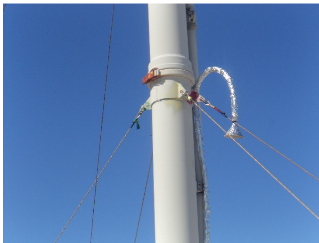
Figure 3. S1 inlet with funnel, insect screening, and temperature insulation attached to the larger-diameter AOS inlet during the calibration period at ENA C1 before deployment at S1.
