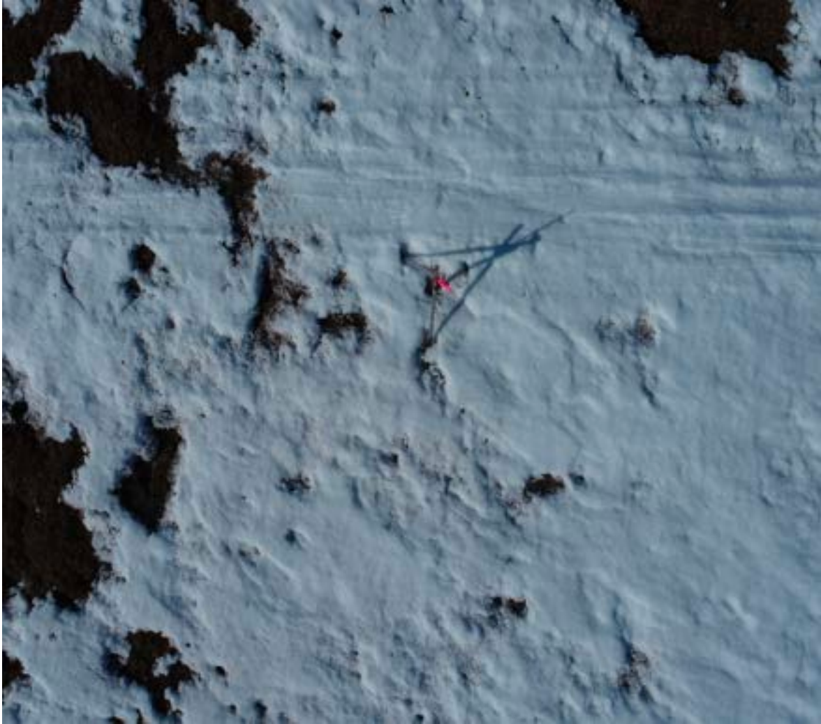
Figure 4. A nadir image of the footprint of the ASD and Kipp and Zonen albedometers. The orange flag is on a small tripod about 1-meter across. The albedometer footprints are about 2-meter in diameter and 1.5-meter south (below) the tripod, which is at the 100-meter midpoint of the 200-meter line shown in Figure 2.
