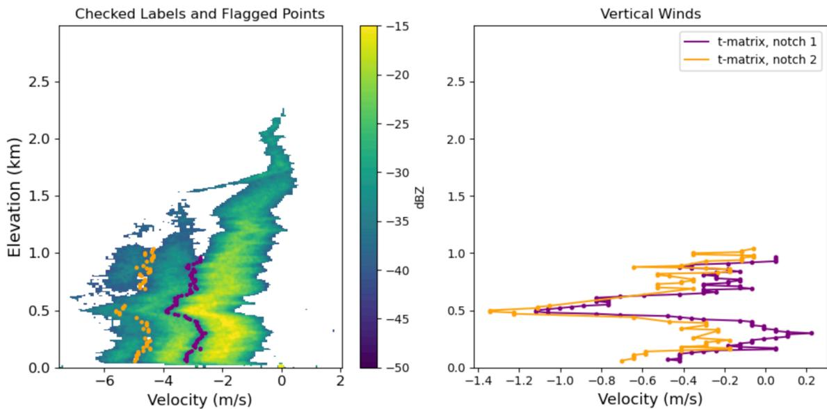
**Figure 4.** A profile of G-band Doppler spectra during shallow cumulus showers with purple and orange dots showing the locations of the first and second Mie-notches (left) and derived vertical air motion from the area of each notch (right).
