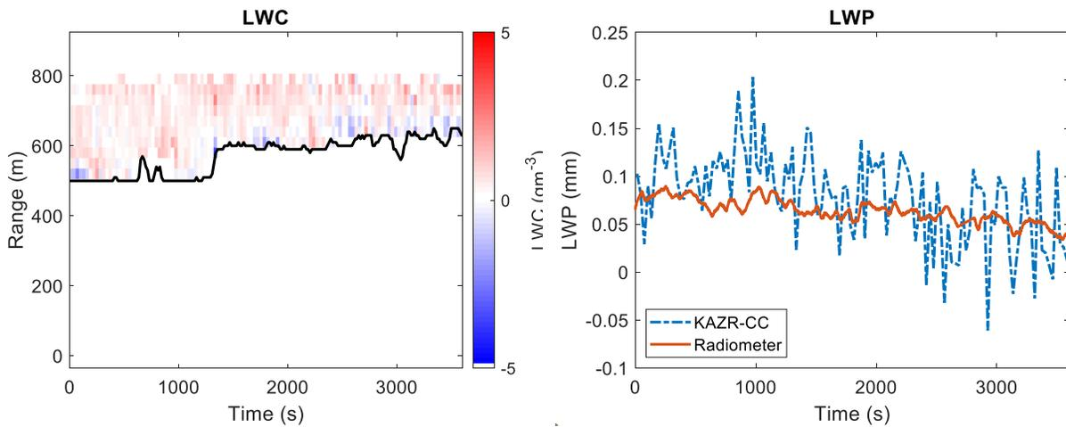
**Figure 3.** Retrieved profiles of liquid water content from the Dual-Frequency Ratio (Ka/G) derived from combining KAZR and CloudCube observations (left). A comparison of the Integrated liquid water path from the radar DFR retrieval and the independent measurement from the microwave radiometer.
