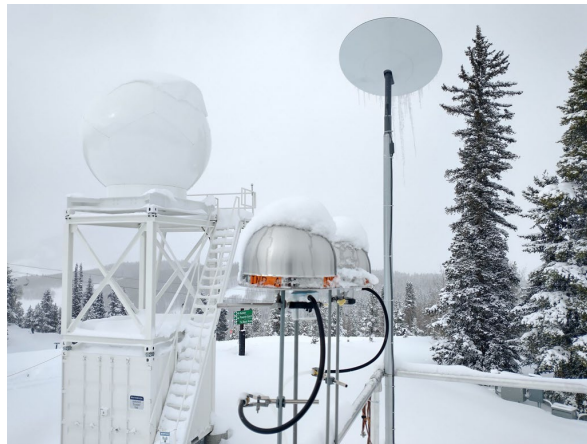
Figure 18. An ice nucleation spectrometer (INS) and an X-band precipitation radar (XSAPR) on Crested Butte Mountain, Colorado for the SAIL campaign in January, 2023. Image courtesy of ARM.
