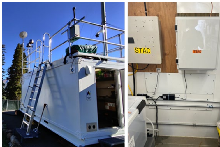
Figure 1. STAC and TBAC deployed at the SAIL AOS site. A separate inlet was installed for particle sampling.
