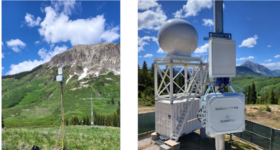
Figure 1. Pictures of the two PM sensors mounted (a) on a platform at M1 in Gothic, Colorado, and (b) on the roof at S2 located midway up Crested Butte Mountain in the Crested Butte Ski Valley.
