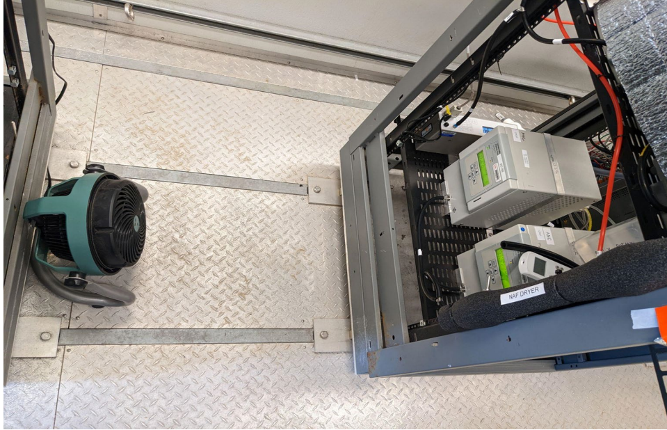
Figure 3. The condensation particle counter-fine (CPCF) and condensation particle counter-ultrafine (CPCUF) inside the ANC AOS of TRACER-ACE, with a small fan directing cooling air to the instruments.
