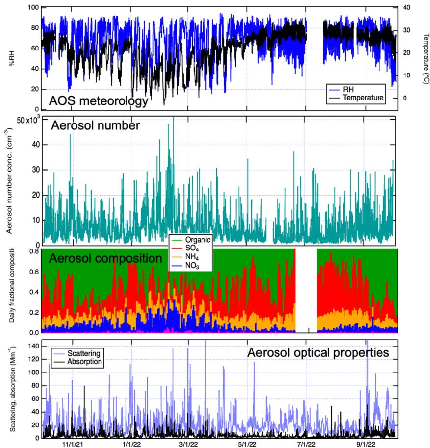
**Figure 9.** Summary of observations from the ARM AOS deployed at the M1 site including the surface-based temperature and relative humidity from the AOS meteorological sensors, aerosol number concentration measured by the SMPS, aerosol composition derived from the ACSM, and aerosol optical properties from the nephelometer (scattering) and aethelomter (absorption).
