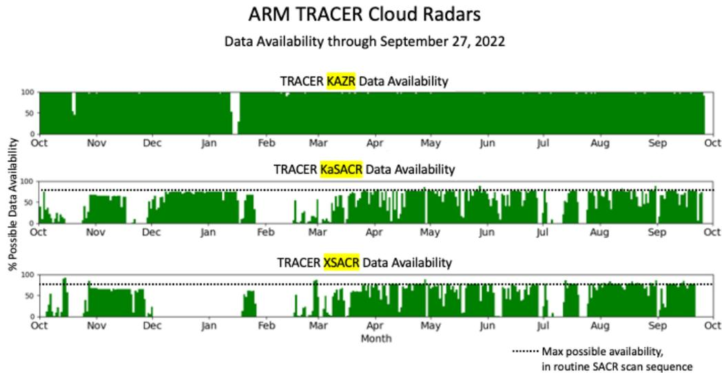
**Figure 4.** Summary of data availability for the ARM cloud radar systems deployed at the M1 site (La Porte, Texas) during the TRACER campaign: (top) Ka-band ARM Zenith-pointing Radar (KAZR), (middle) Ka-band Scanning ARM Cloud Radar (KaSACR) and (bottom) X-band Scanning ARM Cloud Radar (XSACR).
