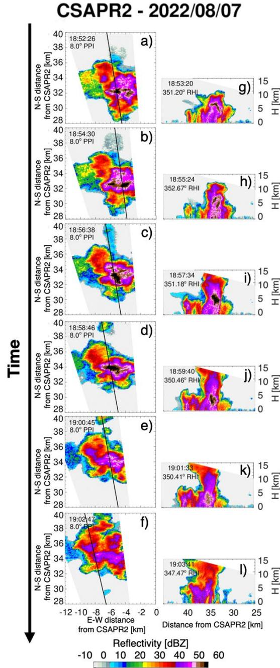
**Figure 7.** Temporal evolution of the 07 August 2022 convective cell between 18:52:26 and 19:03:41 UTC as viewed by (a-f) a CSAPR2 PPI and (g-l) a corresponding CSAPR2 RHI. The black line on each PPI subpanel shows the location of the corresponding RHI. (Lamer et al. 2023).
