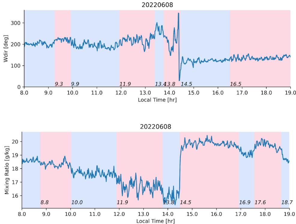
**Figure 10.** Time series of the (top) surface wind direction and the (bottom) water vapor mixing ratio at the M1 ARM site on 08 June 2022 showing the passage of the sea-breeze frontal boundary at about 1430 LT. The blue and pink regions represent time segments identified using the change point detection method.
