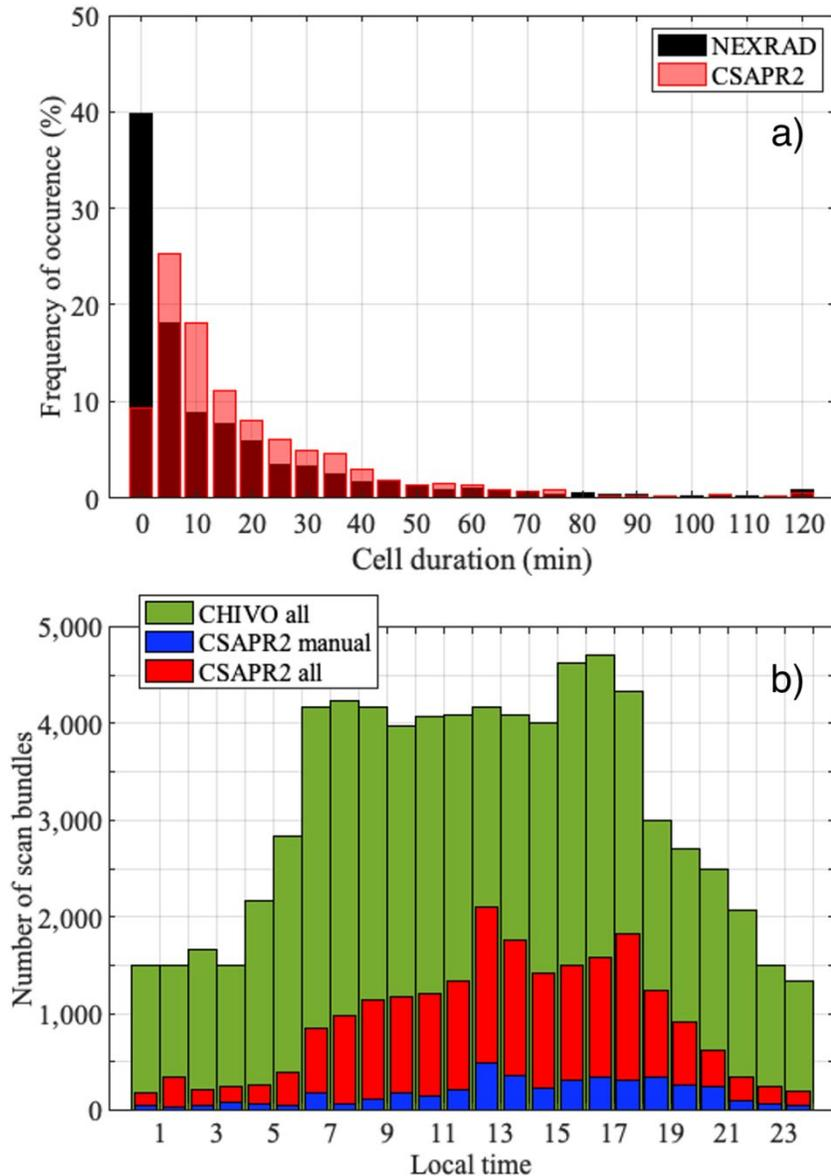
**Figure 8.** a) Distribution of cell duration observed by the KHGX (black bars) and by the CSAPR2 (red bars) during the campaigns and b) number of scan bundles collected by the CHIVO (green bars) and the CSAPR2 (red bars) during the entire campaign and the subset of CSAPR2 scan bundles acquired using online user input to the MAAS framework. (Lamer et al. 2023).
