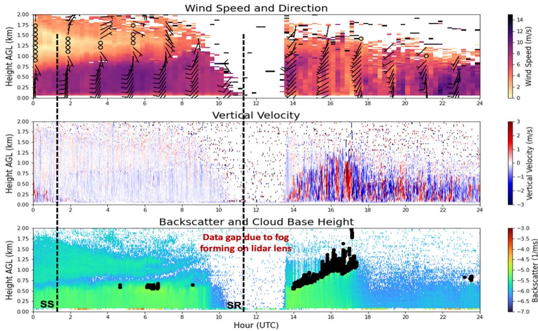
**Figure 2.** Mean wind speed and direction (top panel), 1-Hz vertical velocity (middle panel), and backscatter (bottom panel) collected with the CLAMPS 2 Doppler lidar at the UH coastal site on 07/18/2022. The black dots shown in the back scatter plots indicate cloud base height. The black dashed lines highlight the local sunset (SS) and sunrise (SR) times.
