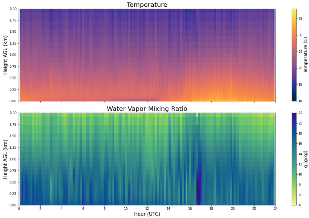
**Figure 4.** Temperature (top panel) and water vapor mixing ratio (bottom panel) retrieved from the CLAMPS 2 thermodynamic profiler data collected at the UH coastal site on 07/18/2022.
