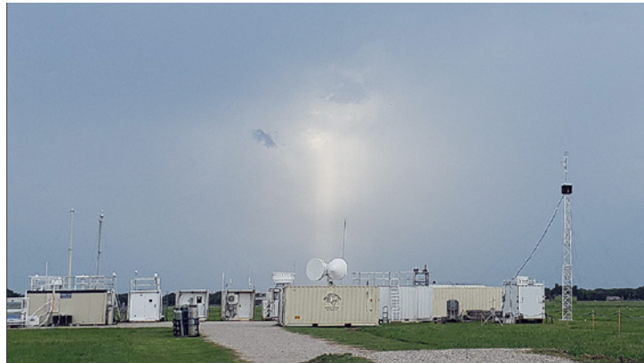
Figure 1. The trailer and flux tower co-located with the aerosol mobile facility during the TRACER campaign. The flux tower is the tower with the black box mounted near the top at the right of the picture. Aerosol instruments were housed in the trailer situated to the left of the tower.
