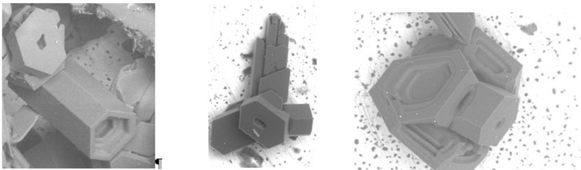
**Figure 4.** Classical single crystals (hexagonal plate and column, left image), planar polycrystal (middle image), and interfused polycrystals (right image).
