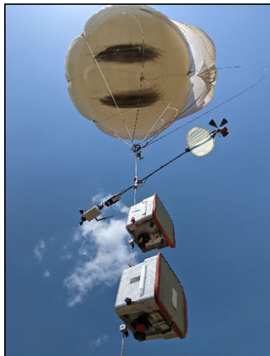
Figure 1. Image of 1-nm CPC onboard the ARM TBS.
