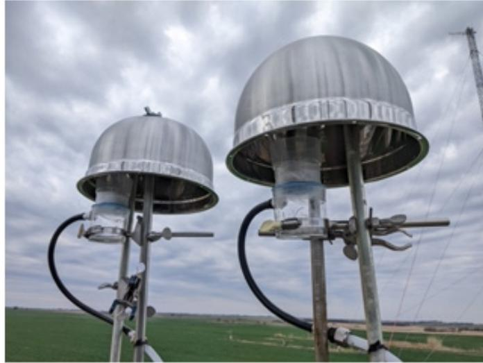
**Figure 2.** Ground-based sampling of INPs at the ARM SGP site. Photo: Darielle Dexheimer, Sandia National Laboratories.
