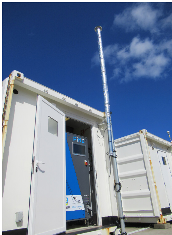
Figure 2. A 5.5-m-height (0.1 m diameter) cylinder-shaped sampling stack inlet was mounted to the instrument container, allowing an intake of particle-laden air by the PINE chamber and other instruments inside.
