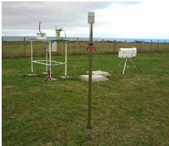
Figure 2. The JCI 131F field-mill (Chilworth, United Kingdom) installed at Graciosa, Azores.
