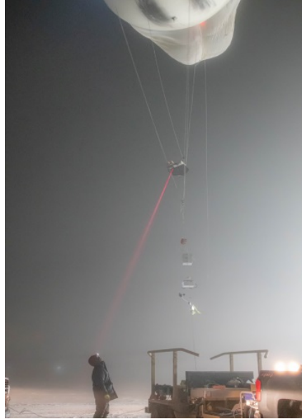
Figure 3. Gondola laser in IF during Flight 2 with instruments along the tetherline on Nov.17.
