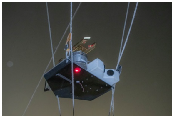
Figure 1. Gondola and CDMS in fog with iced ropes at 04:44 during Flight 2 of IFFExO on Nov. 13.
