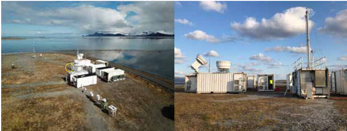
Figure 1. AMF-1 site, looking just east of north from the site at Nordmela Harbor in the left panel, with the filter unit in place atop the AOS trailer (circled) at the start of the sampling period, placed as usual underneath a half-spherical rain hat. Positioning of the filter at 6 m below the AOS inlet intake is more clearly visible in the right figure. These images were at the installation time. Snow covered the site until late May.
