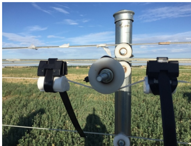
Figure 3. The revised air fiber design in June 2018 and previous setup in 2017. Previous design: the air fiber is directly in contact with the steel wire (the uppermost steel wire in contact with air fiber). Revised design: the air fiber was separated from steel wire by plastic spacers (the middle steel wire connected with air fiber by two black spacers).
