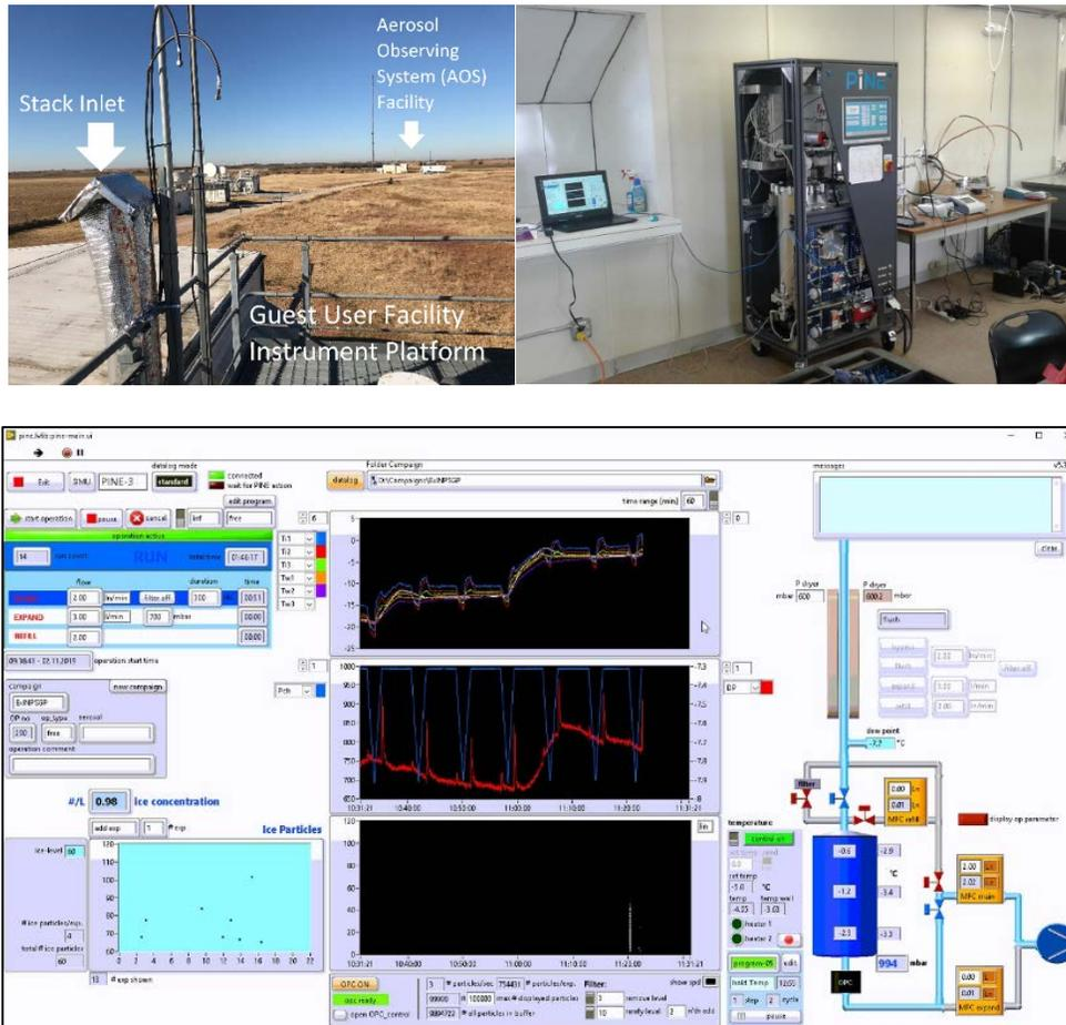
**Figure 1.** The ExINP-SGP campaign was carried out at the ARM SGP Central Facility using the Guest User Facility. A homemade quasi-laminar sampling stack was mounted to the instrument platform (a), allowing an intake of particle-laden air by PINE deployed inside the Guest User Facility (b). For most of the campaign period, the PINE chamber was remotely controlled using the LabView interface through the BeyondTrust remote-access console (c).
