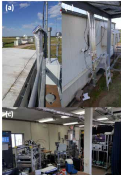
Figure 1. Particle sampling and guest instrumentation employed during AEROICESTUDY. (a) High-volume sampling stack from which instrumentation sampled ambient aerosol particles via a port through GIF housing (b). (c) Guest instrumentation in GIF including PINE, CFDC, MOUDI, SMPS, APS, SP-AMS, and LAAPTOF.
