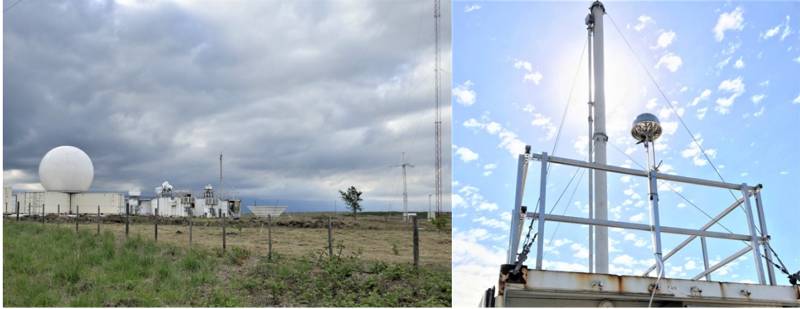
Figure 1. AMF1 site, looking northwest toward the Sierras de Córdoba range behind the trailers (left), with the filter unit in place atop the AOS trailer, underneath the half-spherical rain hat. In this position, it sat only 2 m below the AOS inlet.
