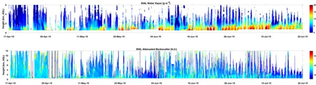
**Figure 2.** Attenuated backscatter from 0-12 km AGL (top) and absolute humidity from 0-6 km (bottom) measured by MPD05 from 17 April–21 July 2019.
