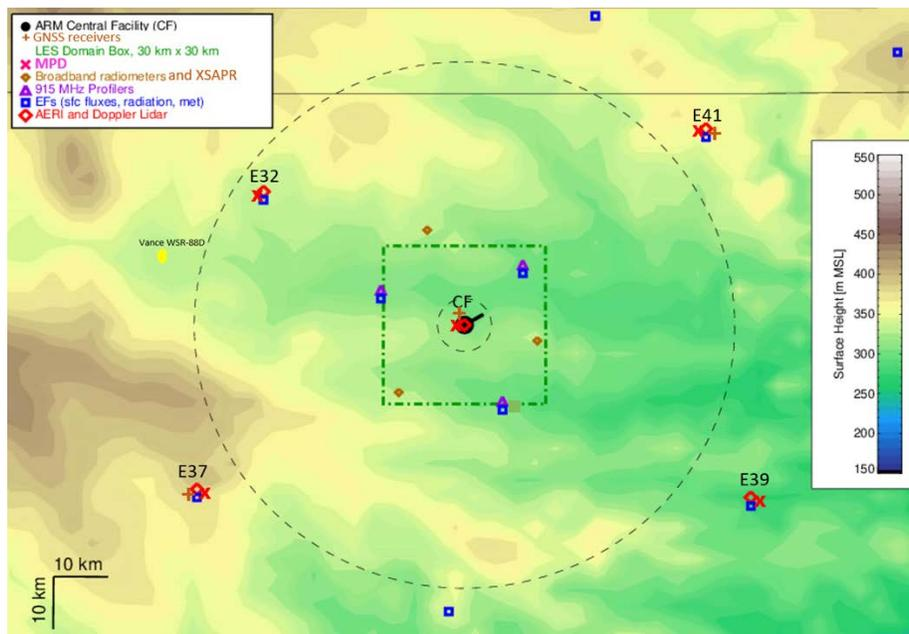
**Figure 1.** Map showing locations of MPD network (pink x's) relative to relevant ARM instruments. Terrain height is shown in color.
