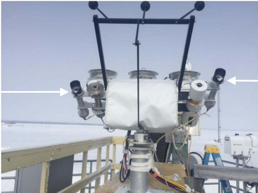
Figure 1. Two Kipp & Zonen CHP1 pyrhemimeters installed at either side of the NSA C1 SKYRAD Solar Tracker.
