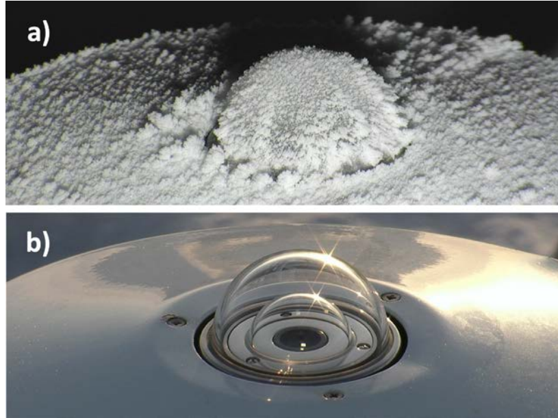
Figure 1. (a) Example of rime ice on January 11, 2018 on the global PSP at the Oliktok Point SKYRAD system. Events such as this were common during mid-winter extending into spring. (b) The same radiometer during non-icing conditions for reference.
